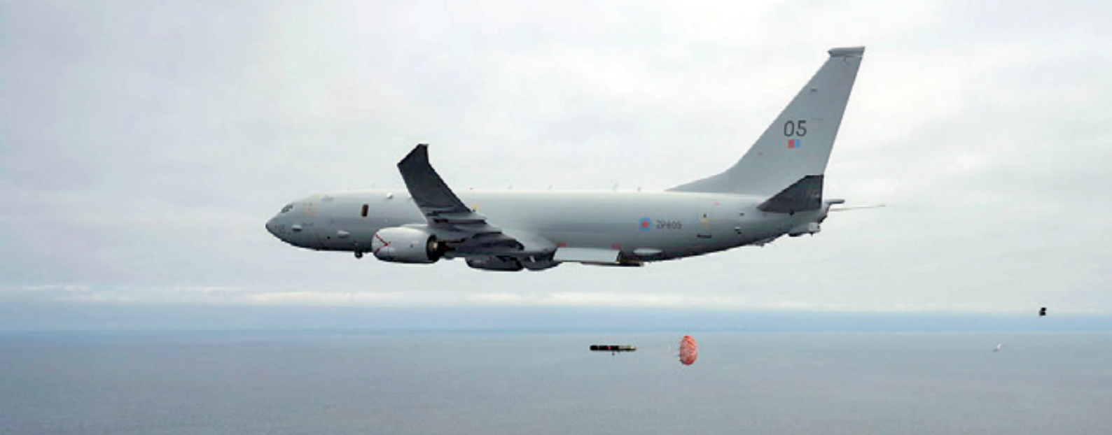
▲ A Royal Air Force Poseidon maritime patrol aircraft releasing a torpedo for the first time on 22 July 2021. In a training flight a Poseidon [P-8A] aircraft dropped a recoverable exercise variant of the Mark 54 Lightweight Torpedo, simulating an attack on a submarine. The MK 54 is an advanced lightweight anti-submarine warfare (ASW) torpedo which can be used in both deep and shallow waters. Photo: UK MoD
