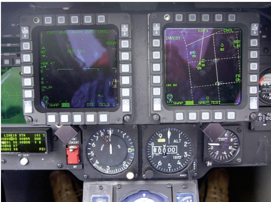
M3 update: A package of software- and hardware-improvements for the F-16A/B Mid-Life Update (MLU). The improvements have been defined and developed since 1998 and includes Link 16 capability. PHOTO: Gøran Bohlin / Scanpix.
