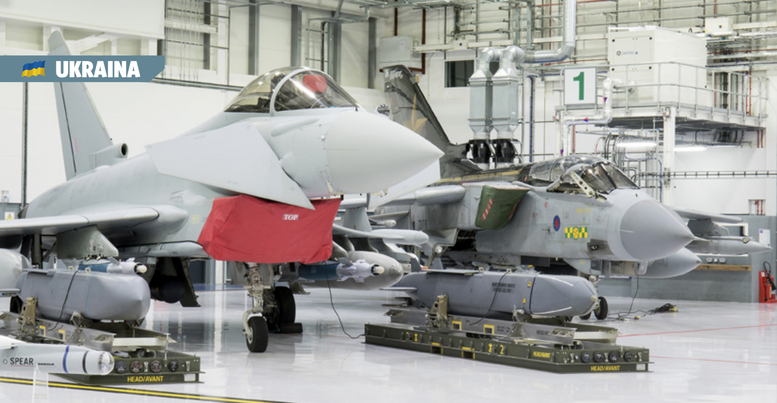
▲ Pictured in a hangar at RAF Marham is a Typhoon (left), pictured with deep strike cruise missile Storm Shadow, air-to-air missile Meteor and the precision attack missile Brimstone. On the right is the recently retired Tornado GR4. Photo: UK MoD
