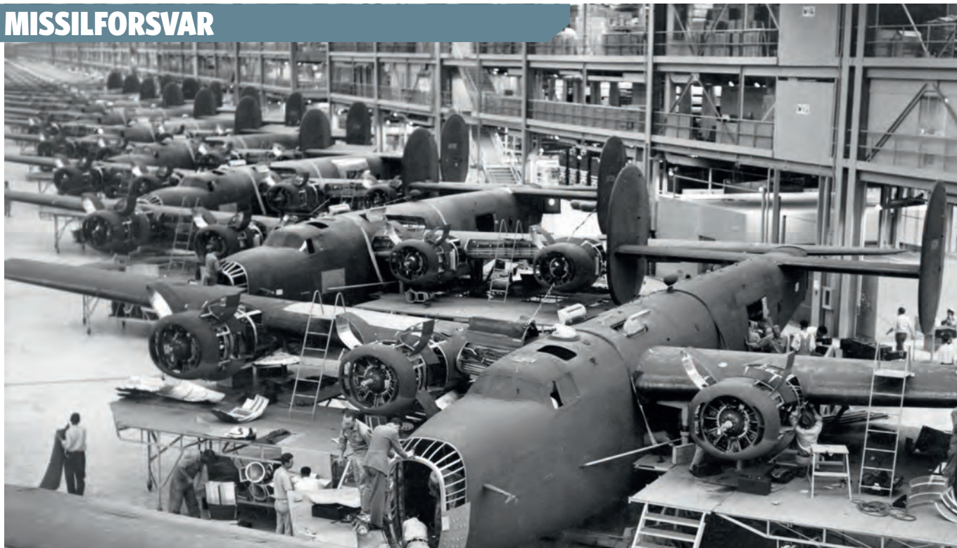
▲ The B-24 was produced in very large numbers. At nearly 19,000 units, it holds the distinction of being the most produced heavy bomber in history, the most produced multi-engine aircraft in history and the most-produced American military aircraft. At the Michigan based Willow Run Bomber plant alone, one B-24 was being produced every 63 minutes at its peak. Photo showing B-24 Liberator bombers nearing completion on the assembly line at the Consolidated Aircraft Corporation plant, Fort Worth, Texas 1942.
