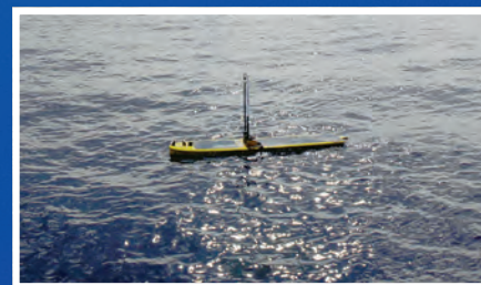
▲ Wave gliders are clever devices which have wave powered propulsion. It can swim or stay in the same position for months. It has several sensors listening below the surface and reports back via satellites or manned/unmanned aircraft. It will be demonstrated during the exercise. Foto: Liquid Robotics
